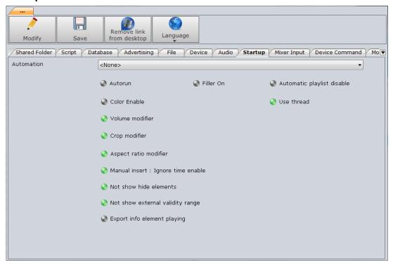
In the configuration of the playout, it is possible to select an automation to execute at the startup.
